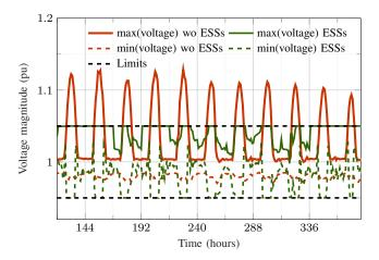
Fig. 6. Evolution in time of the maximum and minimum voltage magnitudes over all the grid nodes before and after ESSs actions for a selected period. Voltage limits are 1 pu $\pm$ 5%.
