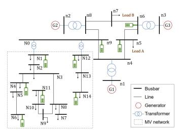
Fig. 1. The case study with an HV and MV grids, conventional generators, loads, and distributed PV generation (not shown). The green icon denotes the location of the batteries (step-up transformers are omitted for simplicity), that is an output of the problem together with their power rating and energy capacity requirements. Load A and Load B refer to aggregated injections of other MV networks.
