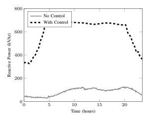
Fig. 3. Reactive power flow on the MV side of the ST before (full line, Case 0) and after the control action (dashed, Case 1).
