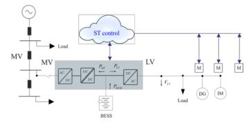
Fig. 1. The considered setup. From the left to the right: a MV network, the smart transformer (ST) with integrated storage and a LV network, whose injections are monitored with smart meters.
