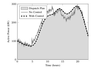
Fig. 2. Active power flow on the MV side of the ST in the case without (full line, Case 0) and with control (dashed, Case 1): in the latter case, it corresponds to the *dispatch plan*, which is computed the day before the operation.
